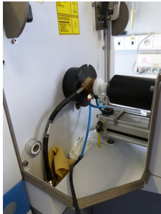
Fig 2: Argon saturation protective bell prototype
