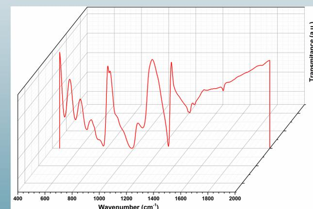
Figure 3: FTIR spectra of AgHAp-PDMS/Si thin films.
