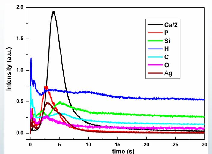
Figure 2: GDOES spectra of AgHAp-PDMS/Si [1].
