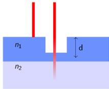
Using DiP for the thickness determination of transparent materials is not straightforward. Indeed, in this case there is no linear relation between the phase shift of the laser beams and the depth of the crater due to multiple reflections at the different interfaces.
