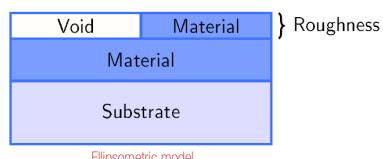
Usually, the **reference technique** for thickness determination of transparent layers is **ellipsometry**.
