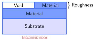
Usually, the **reference technique** for thickness determination of transparent layers is **ellipsometry**.
