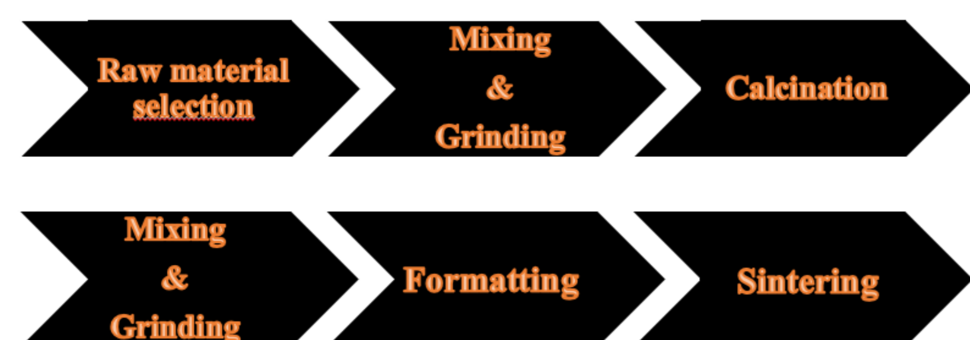
Fig. 2: Principal steps in the fabrication of ceramic.
